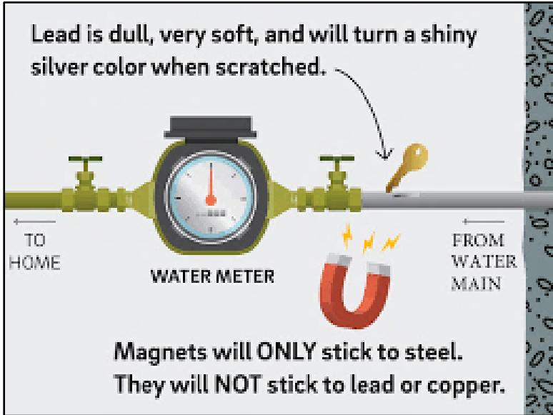
Lead/Lead-lined Water Pipes
